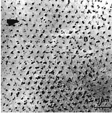
**Figure 1.2:** *One of the first vortex lattice images in a sample of Pb with 4% In at 1.1 K with a field of  $5 \times 10^{-2}$  T.*
