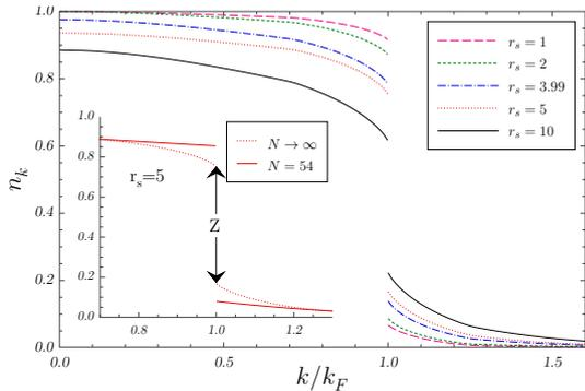
FIG. 3: The distribution  $n(k)$  for HEG, at various  $r_s$ . For small  $r_s$  (large density) the gas is closer to ideal, with step distribution (Ceperley et al.<sup>10</sup>).
